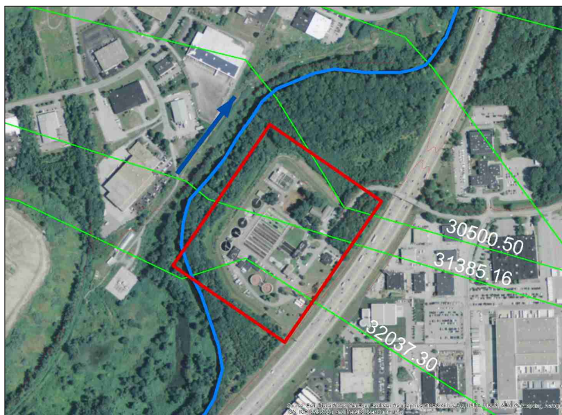
Figure 97: Location of the Warwick Wastewater Treatment Facility, outlined in red. Levee structures are within Warwick Wastewater Treatment Facility perimeter. Green lines show river cross section locations, labeled with cross section identifier numbers. Blue line outlining Pawtuxet River, dark blue arrow showing flow direction of the river.
